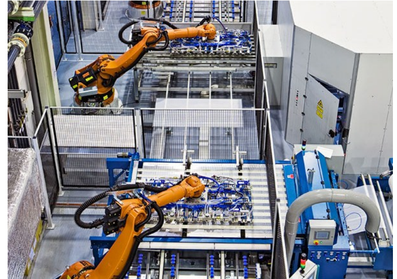
Above: Fully automated production of CIGS solar modules. Below: Roll-to-roll production of thin film.nanosolar.
