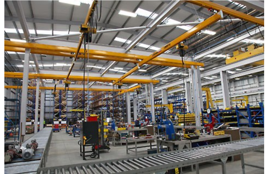
Above: A light crane system is used to increase flexibility at a Siemens advanced manufacturing plant producing power transmission components.
