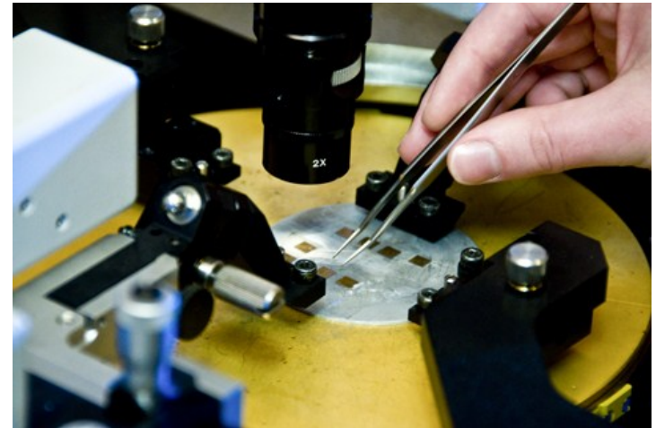
Above: Nanoscale computer chips are arranged under a microscope. Below: Fabricated patterned-photo resists of nanoscale semi-conductors and laser diodes at the Wisconsin Center for Applied Microelectronics.
