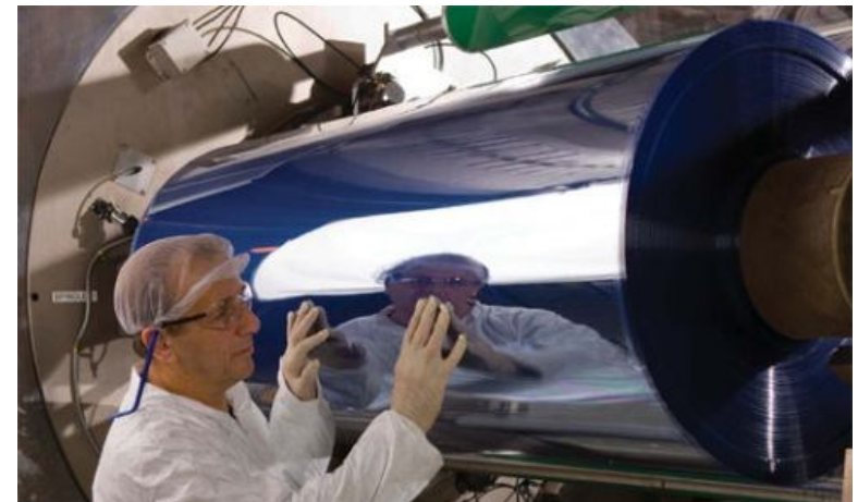
Above: Fully automated production of CIGS solar modules. Below: Roll-to-roll production of thin film.nanosolar.
